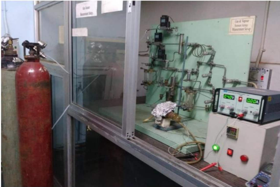
Fig. 4.6. Experimental Setup for TiO 2 -CuO Hydrogen gas sensor.
