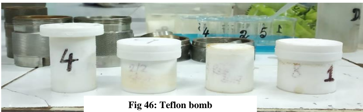
Fig 45: Setup of teflon bomb acid digestion
