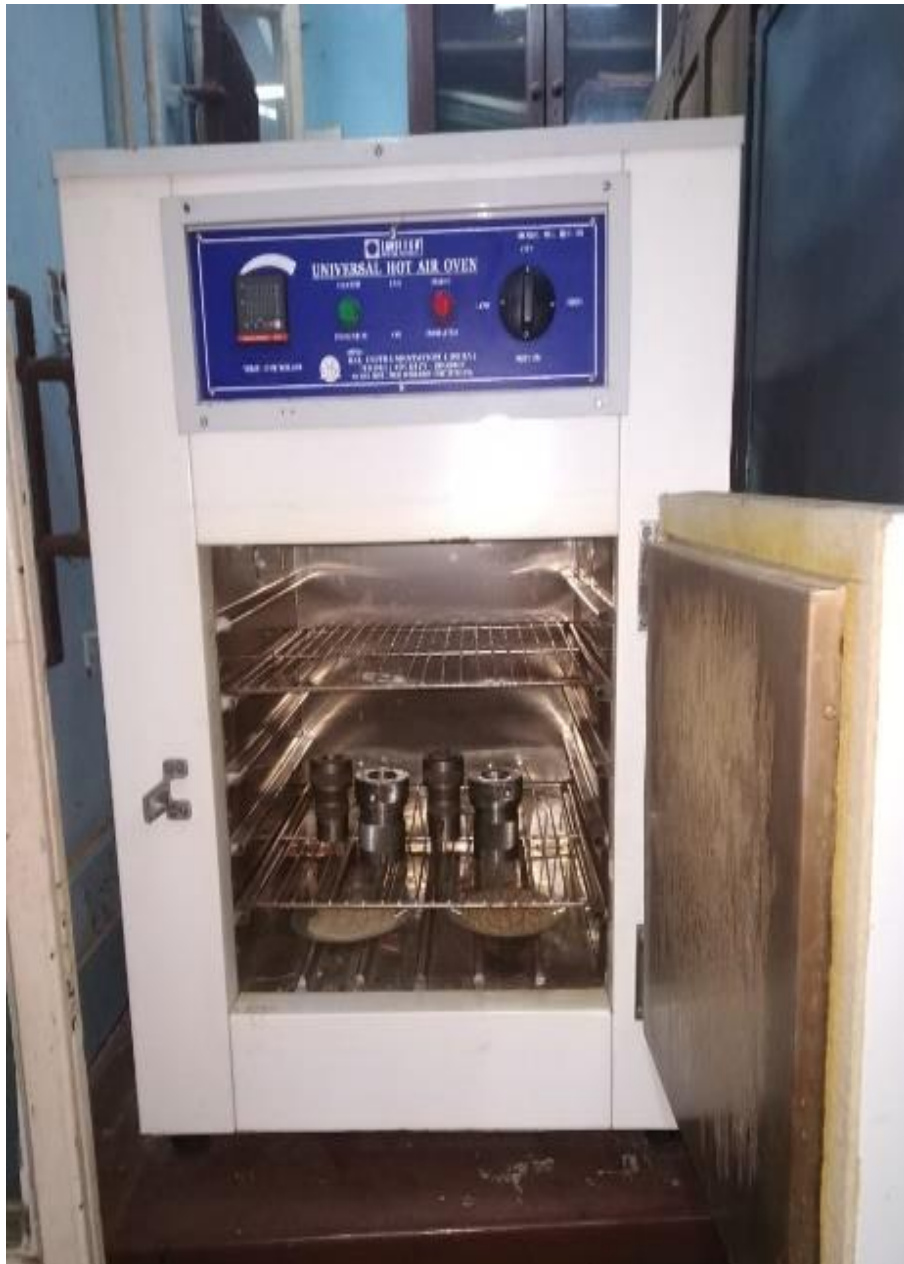
Fig 45: Setup of teflon bomb acid digestion
