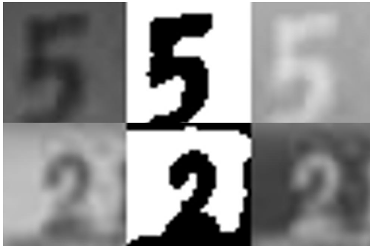
Fig. 9. Preprocessing of image data in SVHN dataset Right-most column showing final output, i.e. all images with darker background.
