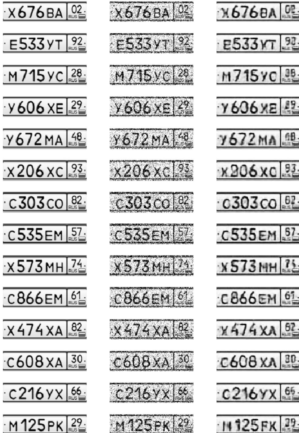
Fig. 23. Denoising output of Autoencoder study II (i) Ground Truth (GT) (ii) noise added to GT (iii) Autoencoder result (proposed model) (by column)
