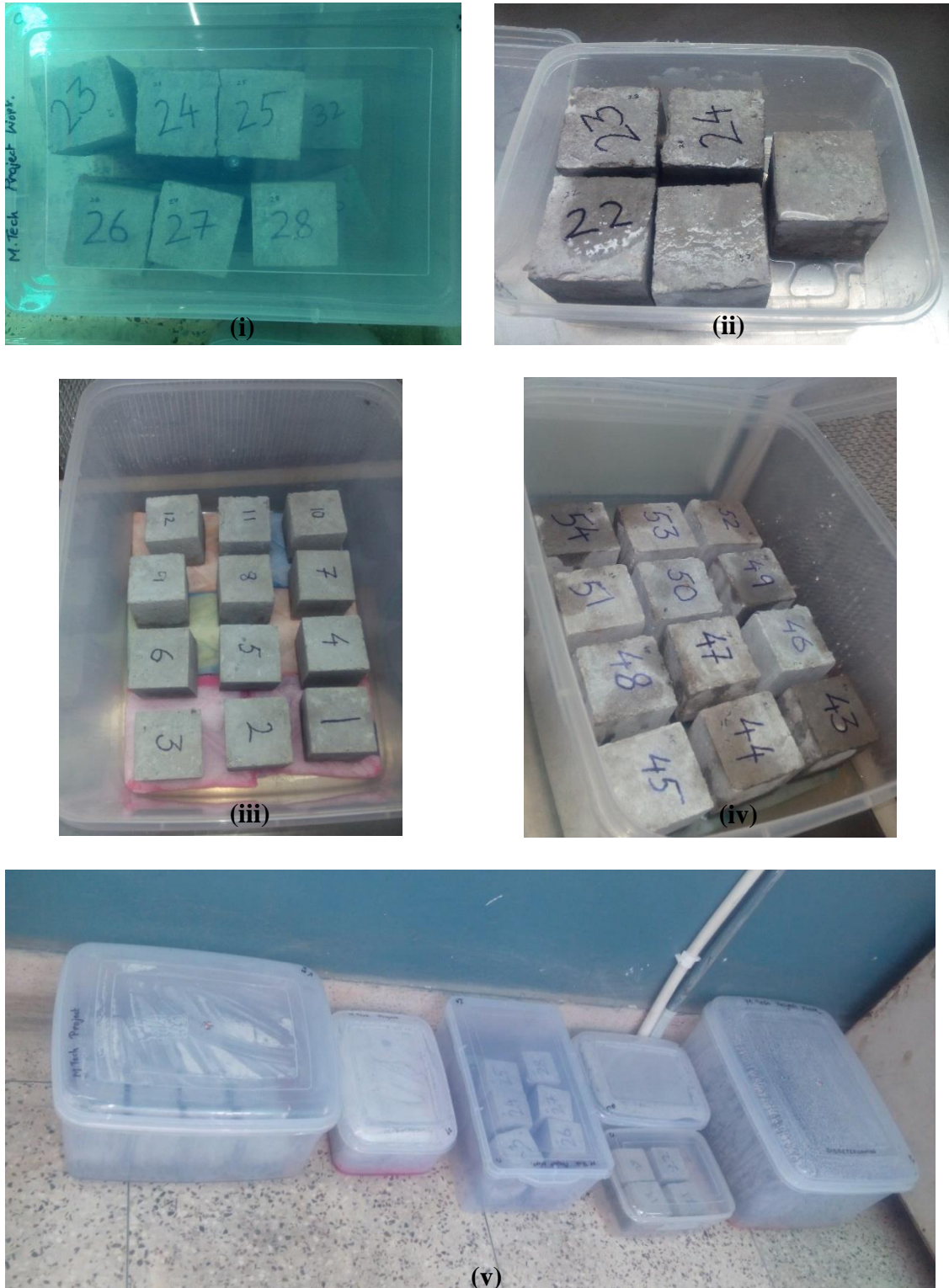
Figure 8: (i)Control set-up (ii)Positive Control set-up (iii)Biodeterioration set-up (iv)Prevention set-up (v)The Final Experimental Set-up arrangement.
