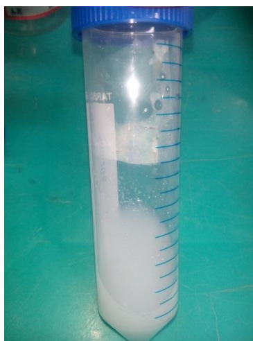
Figure 4: The aqueous milky white coloured Nanoparticle coating after the mixing of the binder, nanopowder and water.
