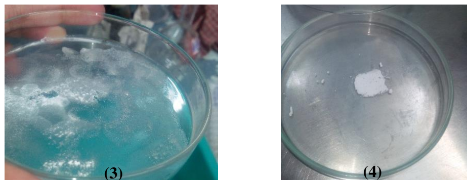
Figure 3: The 4 combinations of binder, silicon oxide nanopowder and distilled water after 48 hours of drying (1) Ratio-1 : 0.1 : 2 (2) Ratio-1 : 0.5 : 2 (3) Ratio-1 : 1 : 2 (4) Ratio-1 : 5 : 2.
