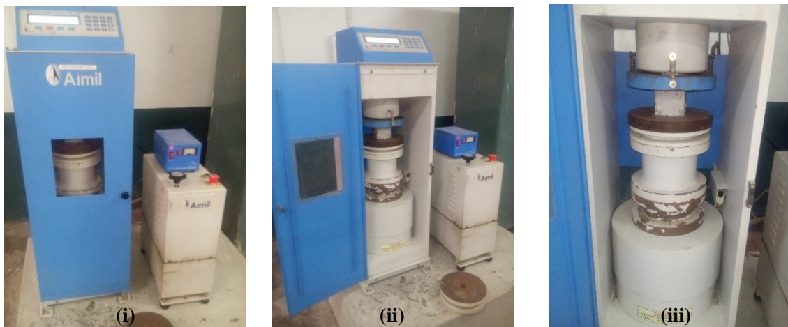
Figure 12: (i) and (ii) :Universal Compressive Strength Test Machine (iii) Concrete cube placed between the spherical plattens for strength test.
