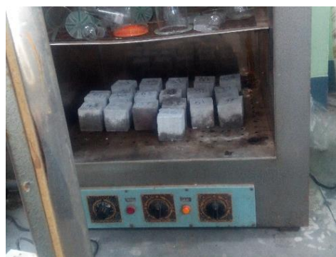
Figure 6: Nanoparticle coated Concrete Cubes in hot air oven after 4 days of drying at 40°C.
