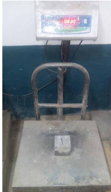
Figure 10: The weight of a concrete cube being measured in the weight balance.
