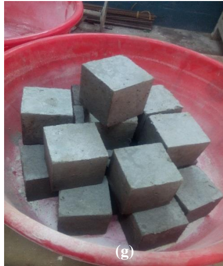
Figure 5: Concrete Cubes preparation : (a)Cement, sand and stone chips mixed in a ratio of 1: 1.5 :3 (b)Water added to obtain the concrete mix (c)Cubic cast iron moulds (d)Concrete poured and leveled in cast iron moulds (e)After drying overnight (f)Cubes submerged in water for curing of 28 days (g)Concrete cubes after curing and 3 days of drying.
