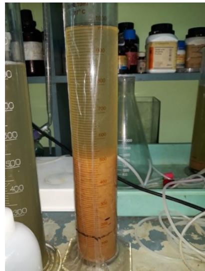
Fig. 5.4- final MLSS volume (After 2 days)
