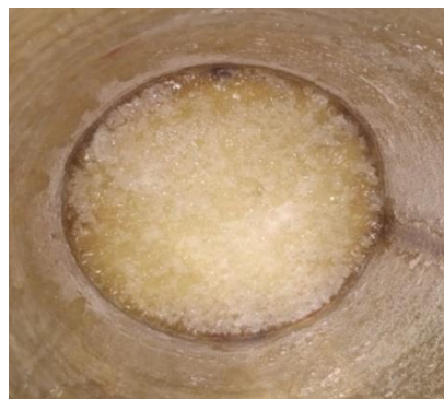
Fig.34. Crystallization of salts for the process with PP membrane after 4 hours
