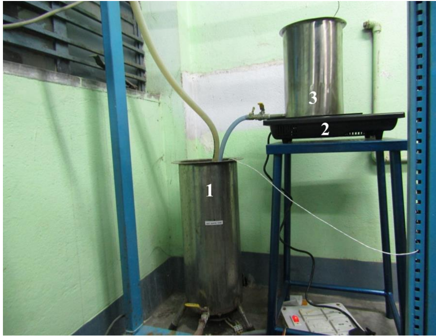
Fig.20. DCMD Reheating equipment (1) heater and reservoir for hot side feed (2) inductive heating system (3) reservoir for cool brine reject.
