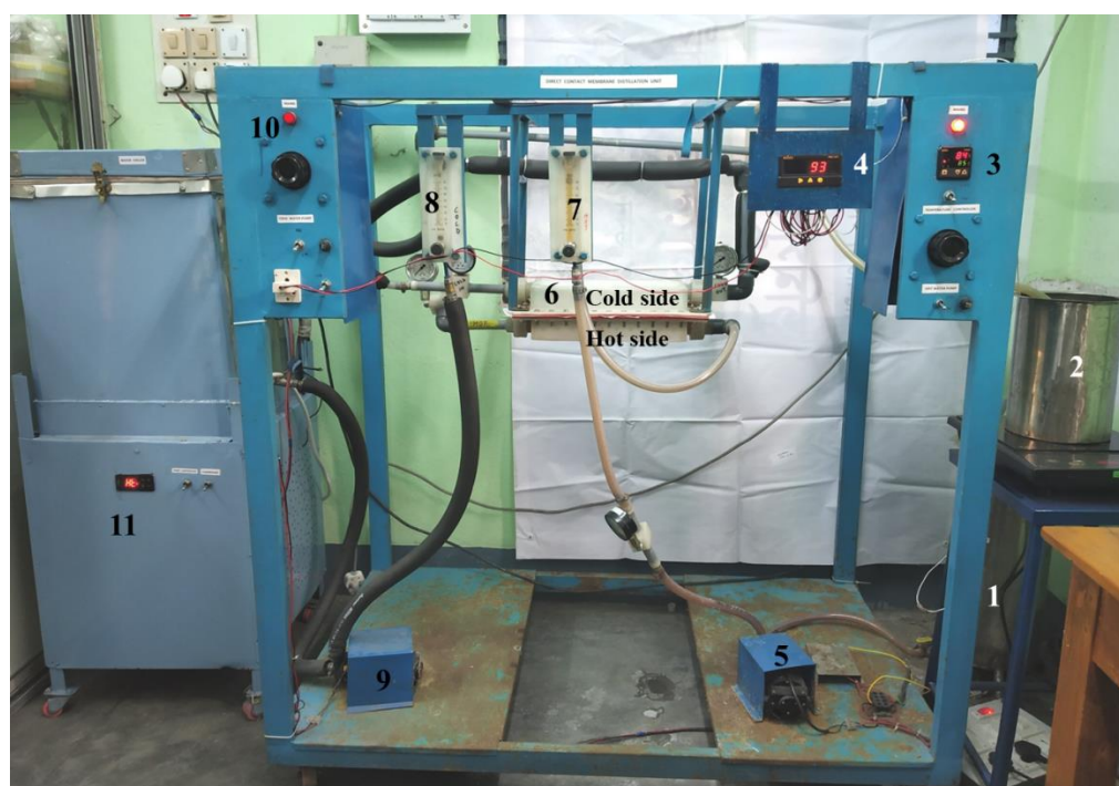
Fig.16. DCMD equipment used in this study (1) heater and reservoir for hot side feed (2) heater and reservoir for reheating of cool brine reject (3) temperature controller for hot side feed and hot pump regulator (4) temperature controller for reheating (5) Hot feed pump (6) DCMD module (7) Hot side feed flow meter (8) Cold side flow meter (9) Cold side pump (10) Cold pump regulator (11) Cold side temperature controller and chiller
