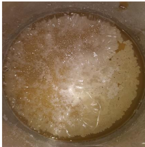
Fig.32. Crystallization of salts obtained in the process with 0.22 µm PVDF
