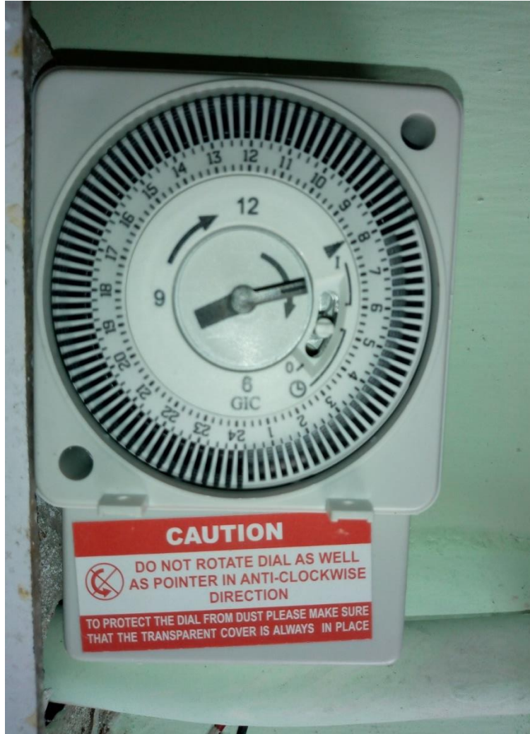
Fig 17 - Timer used in the experiment aligned with warm white light 4000K switched on from 12:00am to 8:00am
