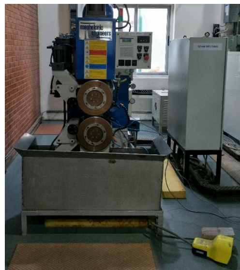
Figure 7.4. Arrangement of Seam welding
