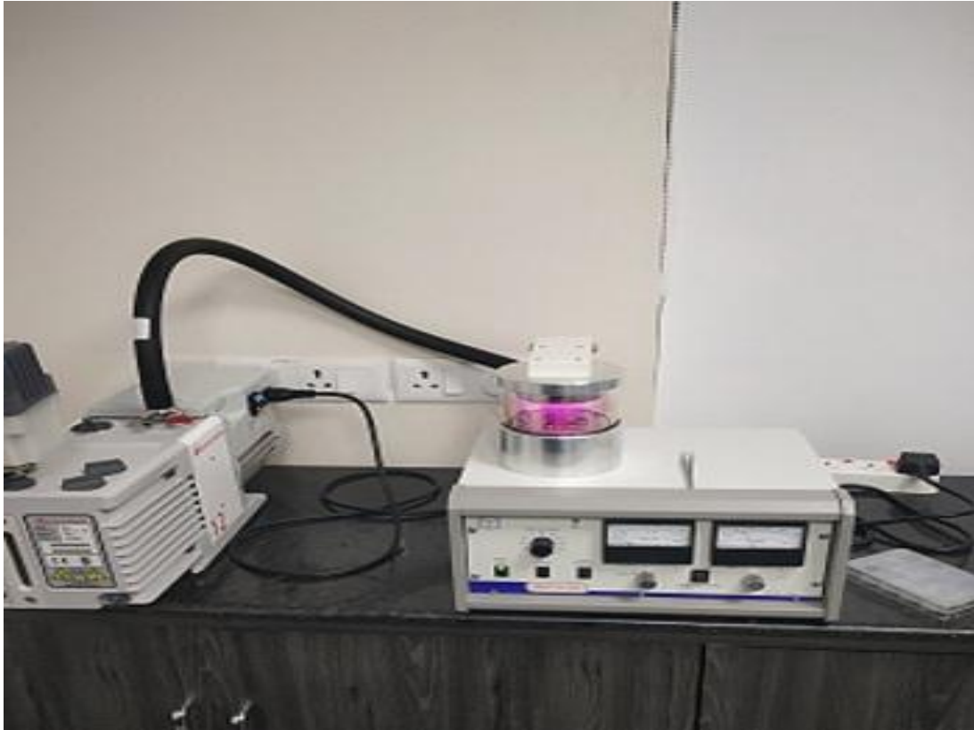
Figure 7: Platinum coating of stubs during Scanning electron microscopic study
