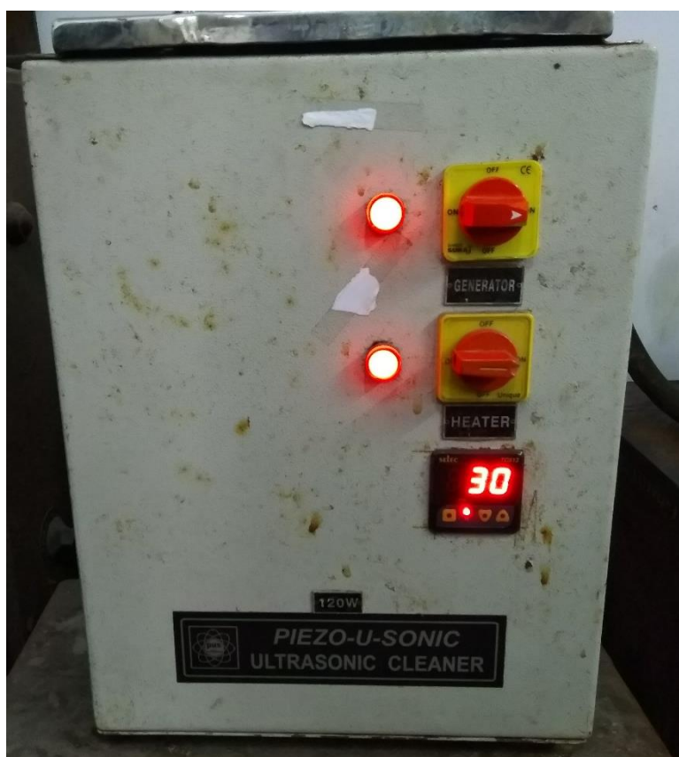
Figure 3.2: Ultrasonic Cleaner is used for heating and drying after formation of gel
