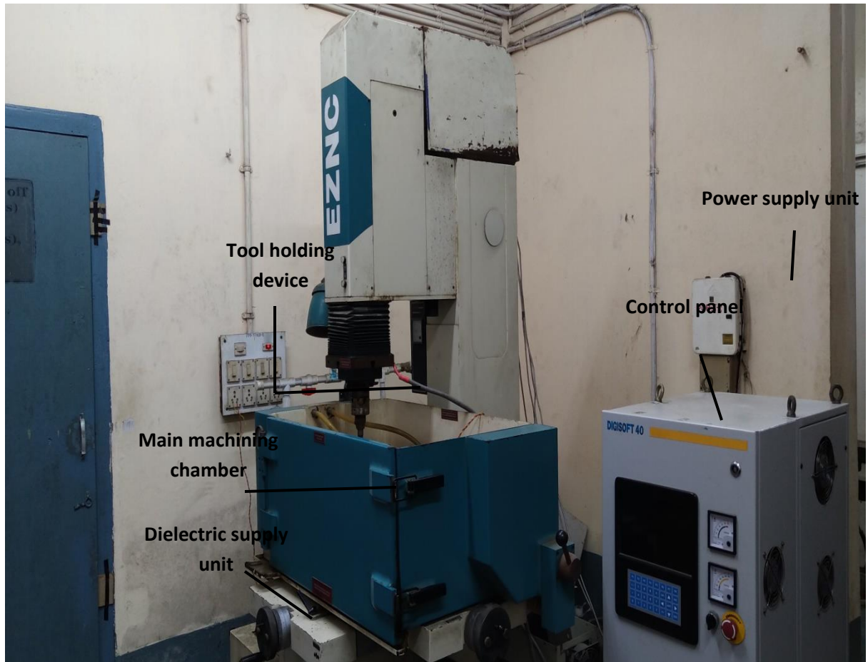
Fig.3.1. Photographic view of S-35 ZNC Die-Sinking EDM Machine
