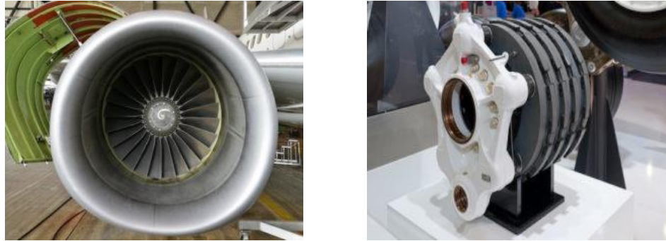
Fig1.4. Aircraft engines and braked made of ceramics
