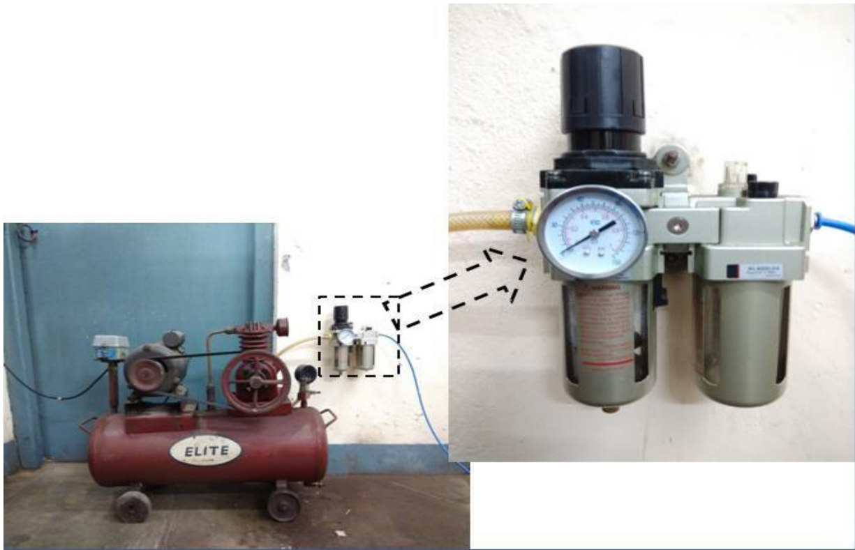
Fig. 3.5. Moisture separator and pressure regulating Unit
