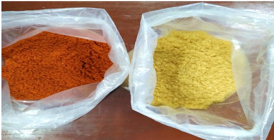
Fig 7.1: Anionic resin and cationic resin
