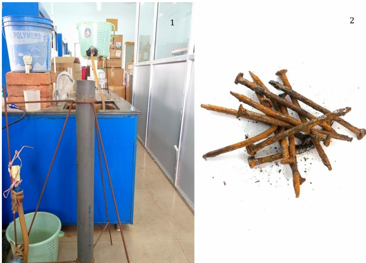
Fig 7.16: (i) Experimental set up in laboratory (ii) rusted iron nails which are used for adsorption.
