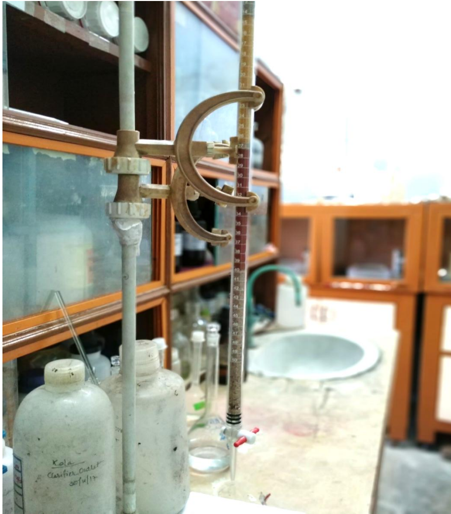
Fig 7.3: anionic-cationic resin burette filter
