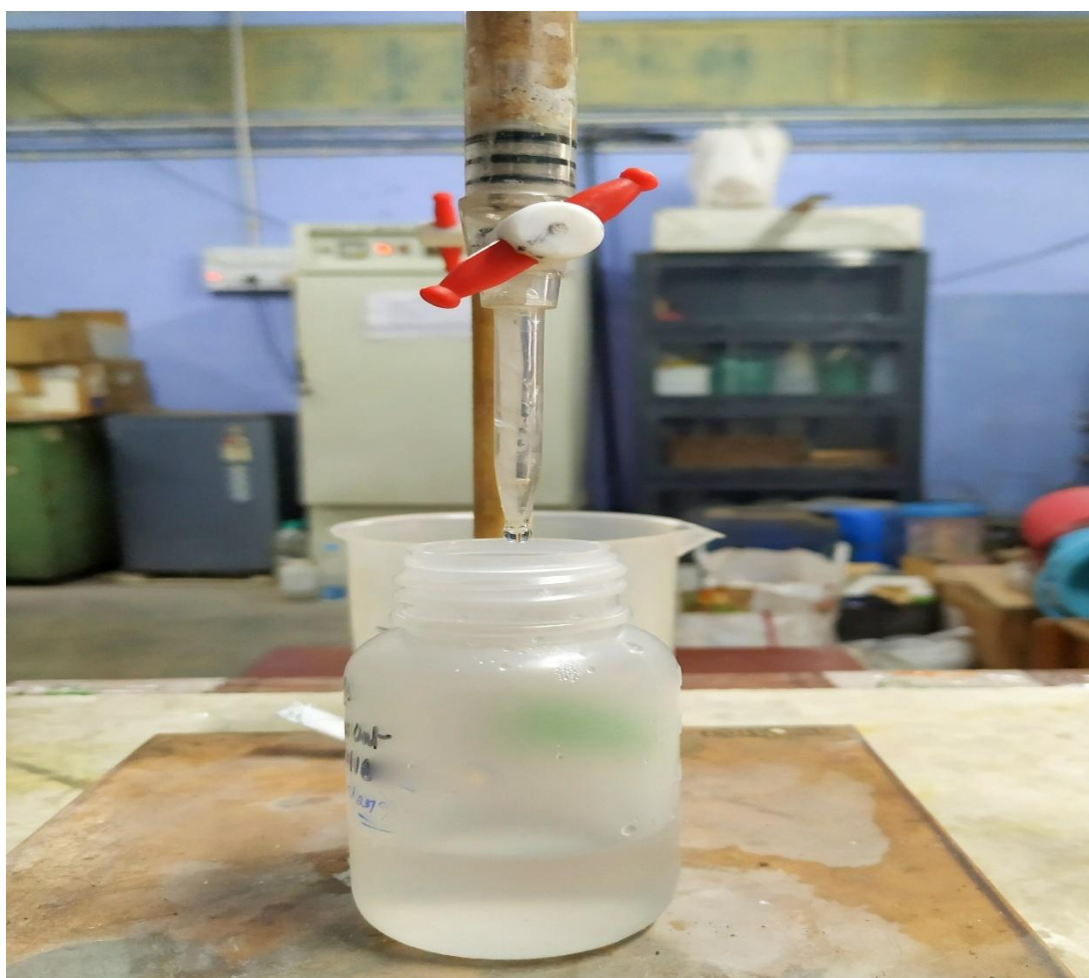
Fig 7.6: Sample collection from cationic resin filter outlet
