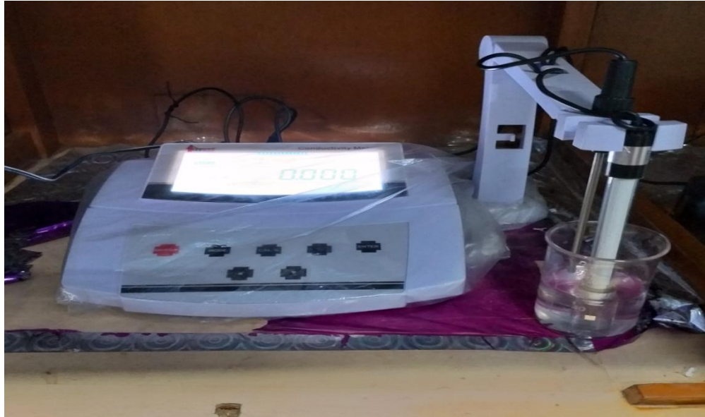
Fig 6.6 Conductivity meter for measuring the TDS & EC
