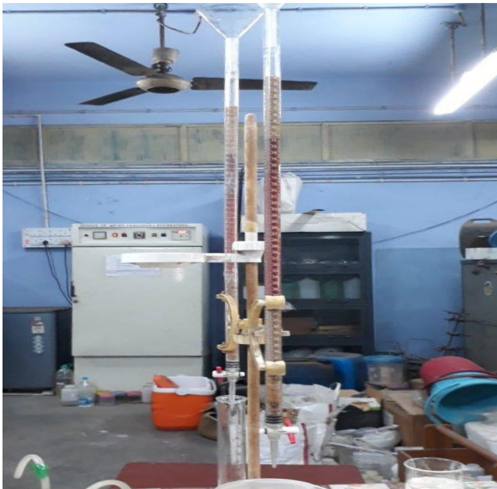
Fig. 7.11: anionic resin burette filter
