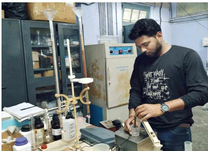
Fig 5.2: Testing in ion meter to determine concentration of fluoride
