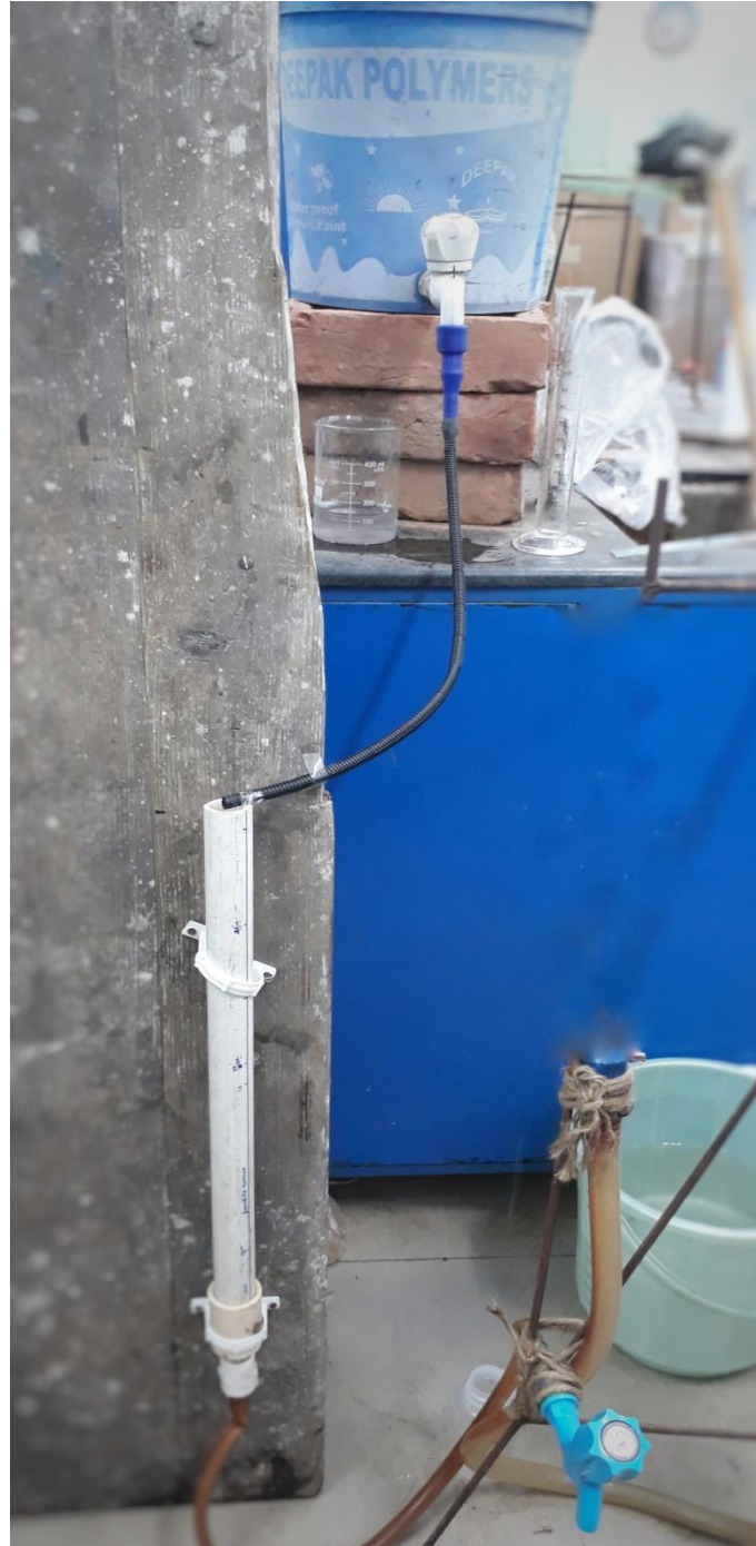
Fig 6.10: Experimental Set-up for adsorption method using Activated Alumina
