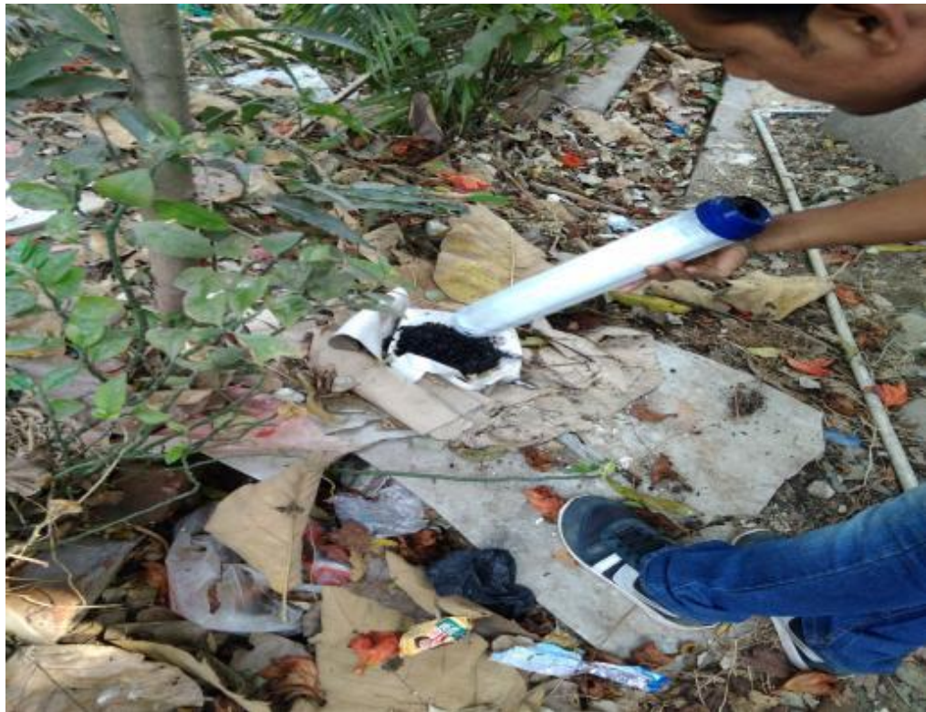
Fig. 62: Removing old GAC after three days of operation
