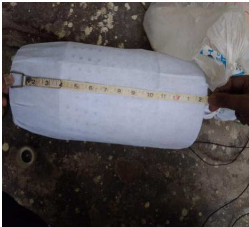
Fig. 67: Perforated pipe covered with cloth filter
