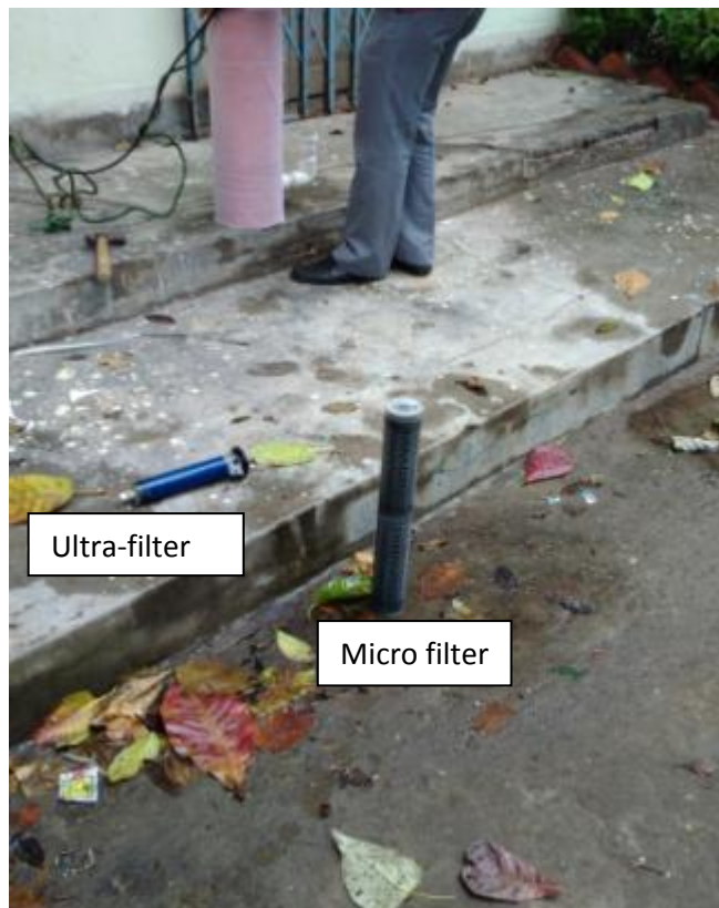
Fig. 30: Condition of micro filter & ultra filter after 3days
