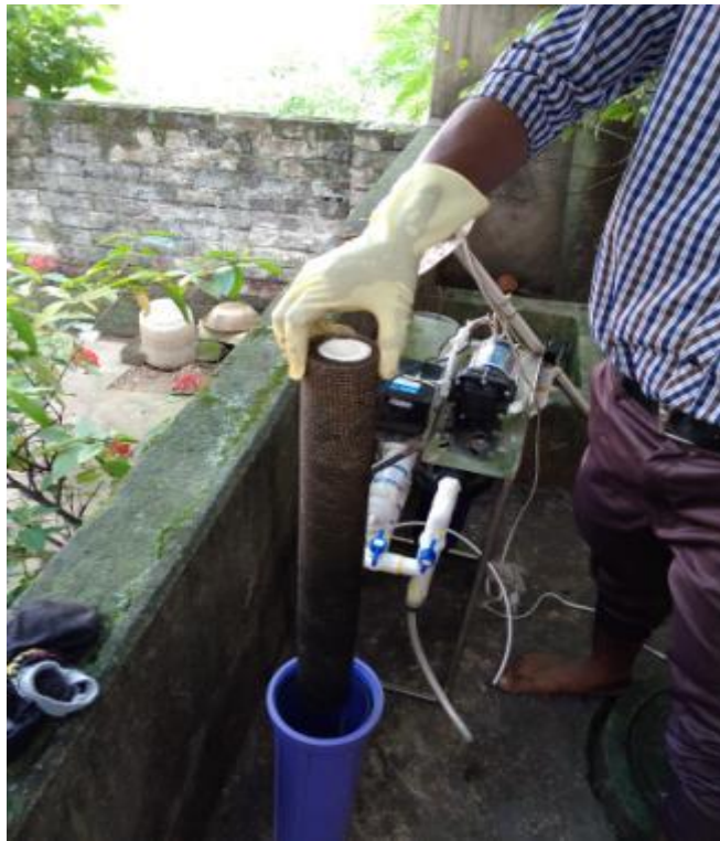
Fig. 13: Micro filter after three days of running previously it was white
