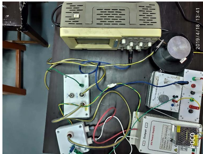
Fig. 5.6. Experimental Setup for PDC measurement.
