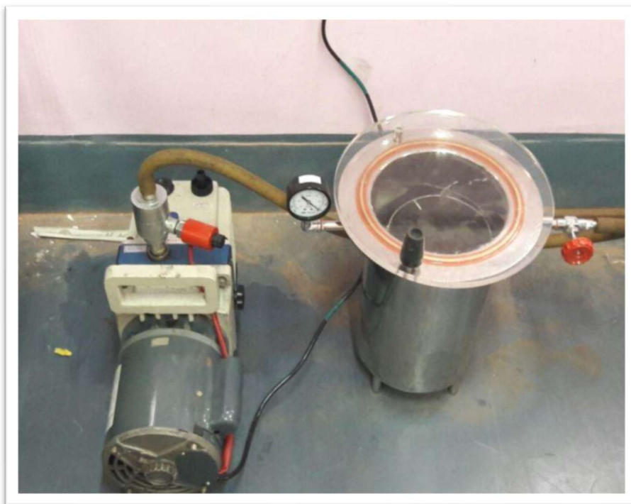
Figure 4.8: The Degassing unit
