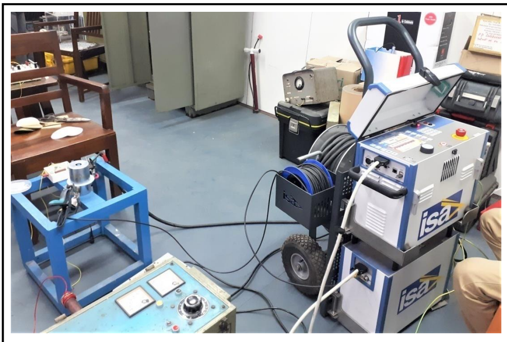
Fig. 5.30. Experimental setup for tan-delta measurement.
