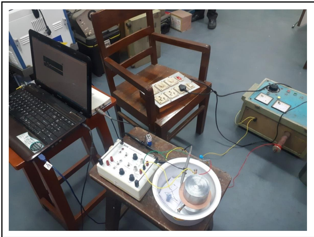
Fig. 5.23. Experimental setup for the measurement of the signal of known charge magnitude using PD calibrator.
