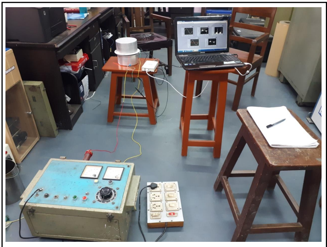
Fig. 5.25. Experimental setup for obtaining the PRPD pattern.
