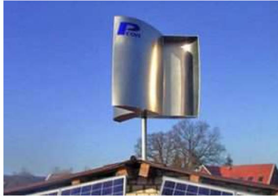
FIG2.8 :- savonius rotor structure
