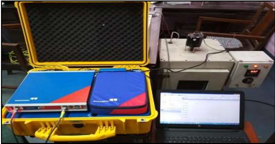
Fig.4.8. Experimental setup for PDC measurement of XLPE cable using DIRANA
