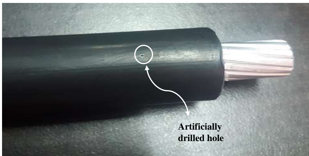
Fig. 4.6. Artificial defect created on XLPE insulation surface
