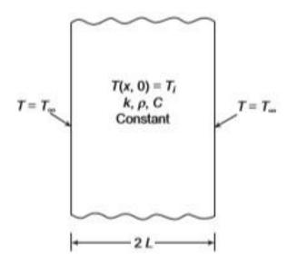
✓ The case of a hot infinite plate of finite thickness 2L, is suddenly exposed to an atmosphere of temperature  $T = T_{\infty}$ .
