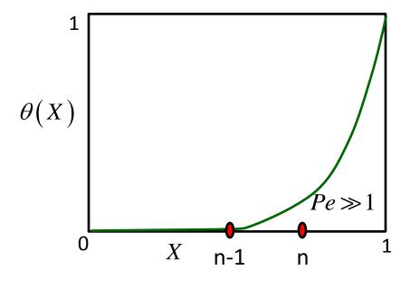
When Pe is large,  $d\theta/dX$  is nearly zero at X=0.5. Thus, the diffusion is almost absent. The upwind scheme always calculates the diffusion term and thus overestimates diffusion at high Peclet numbers. This is called False Diffusion.
