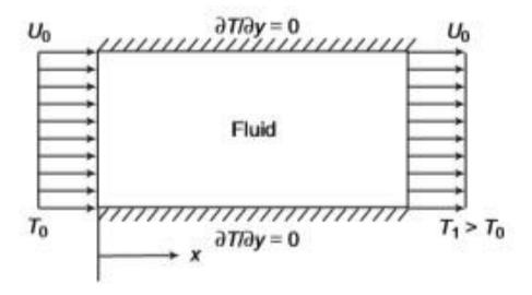
Convection diffusion problem for slug flow where the combined influences of steady axial convection and diffusion is examined. The fluid is flowing with a velocity  $U_0$  and is subjected to specified temperatures as follows:
