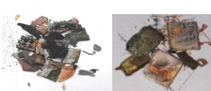
Figure 7.1: Solid Residue of (a) FR-2 and (b) FR-4 WPCB steam gasification
