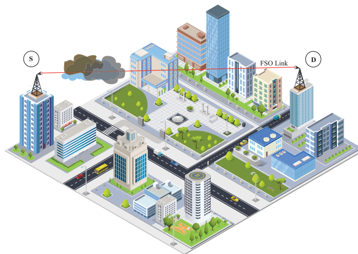
FIGURE 1.2: A typical free space optical communication system.
