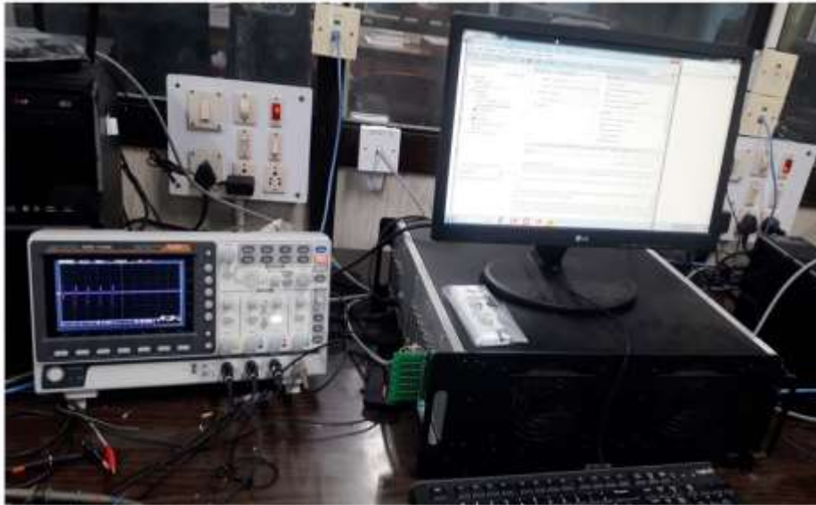
Fig. 6.9. OP5600 Set-up for real time application of the proposed control scheme.
