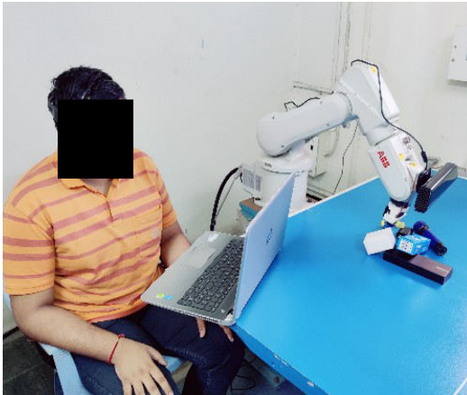
Figure 4.9: Step1: The robot is at it's initial position and the subject uses his motor imagery and P300 to rotate the robot arm and select the desired object respectively.
