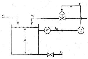
Draw the block diagram of the level control system. For a unit step change in disturbance, find the expression of steady-state error or offset under proportional control.
