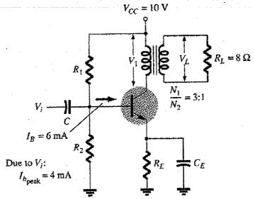
4) Calculate the input impedance, output impedance, voltage and current gain for the circuit given below.
