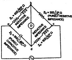
II) Find the value of unknown resistance and capacitance for the balanced bridge while a 50Hz supply is applied across a-c terminal.
