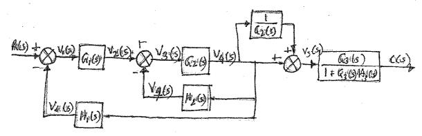
Draw the corresponding Signal Flow Graph and validate the result obtained by Block Diagram Reduction using Mason's Gain Formula.10+10
