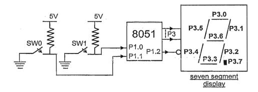
Write an appropriate program to sense the switches. If SWO is closed a '0' will be displayed. If SW1 is closed a '1' will be displayed. If both the switches are closed an '8' will be displayed. For no key press, nothing will be displayed.
