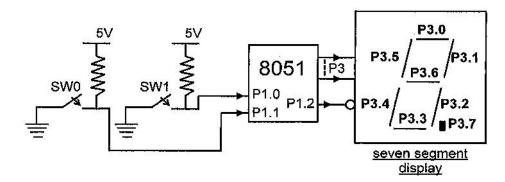
Write an appropriate program to sense the switches. If SW0 is closed a '0' will be displayed. If SW1 is closed a '1' will be displayed. If both the switches are closed an '8' will be displayed. For no key press, nothing will be displayed.
