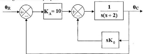
Determine the derivative feedback constant, K<sub>0</sub>, which will increase the damping ratio of the system to 0.6. What is the steady state error resulting from unit ramp input for this new setting of derivative feedback constant.
