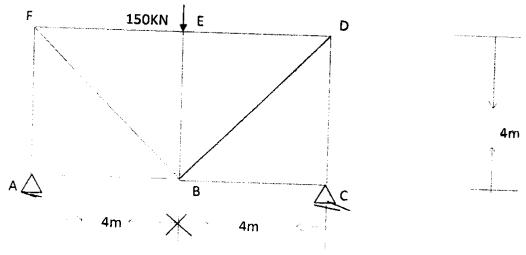
2. A) Determine the Horizontal deflection of Point C in the frame as shown in Figure. Take  $E=2X10^5 N/mm^2$ .  $I=30X10^6$ .[ 10+10=20.]
