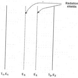
Hint: Without shields:  $Q_{12} = (F_g)_{12} A_1 \sigma_b (T_1^4 - T_2^4)$ .
