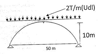
6. CO6: A simply supported beam is loaded as shown. Section of beam is 450mmX350mm
