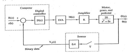
(b) Design a digital controller D(z) to attain a steady state error less than 0.01 for unit ramp input and to ensure stability of the entire system with  $G(s) = \frac{1 - \exp(-Ts)}{s(s+1)}$  and T=0.1 sec.
