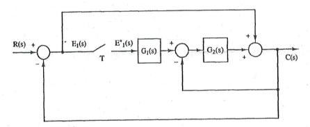
2. (a) Evaluate the closed loop transfer function of the following antenna control system with D(z) = 1, T = 0.05 s, K = 20.
