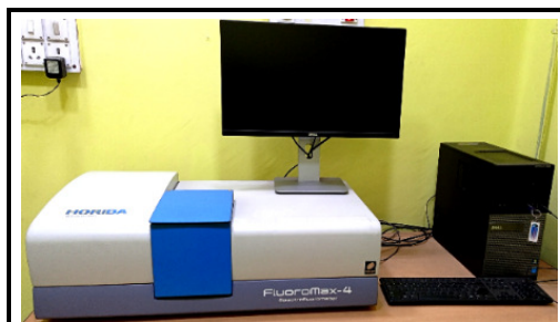
Figure 4.10. Typical steady-state fluorescence emission Spectrophotometer installed in our laboratory.
