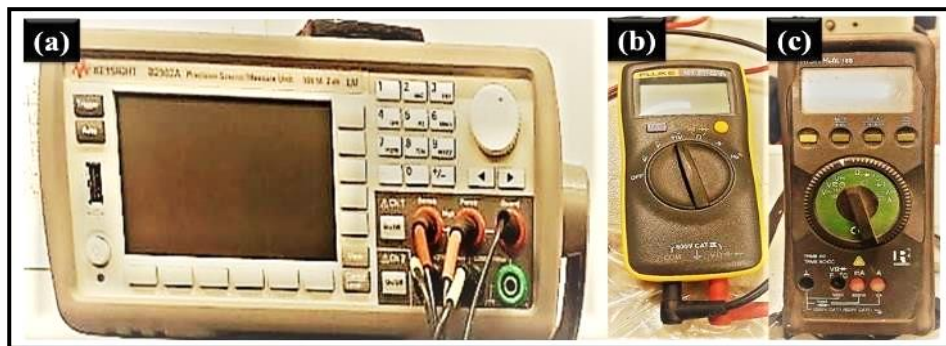
Figure 3.11: (a) Electrometer and (b & c) digital multimeters
