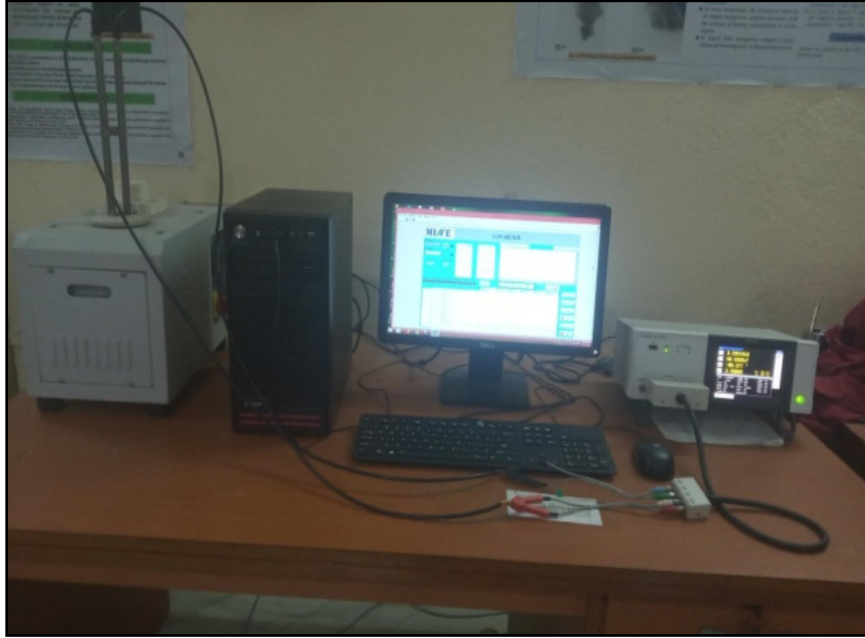
Fig 2.11 Experimental set-up of LCR meters.
