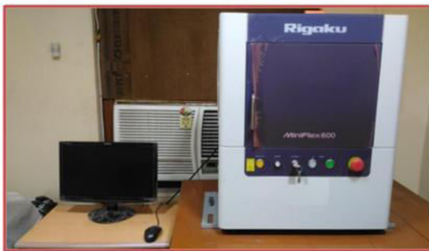
Fig 2.5 Photograph of X-ray diffractometer experimental set-up.
