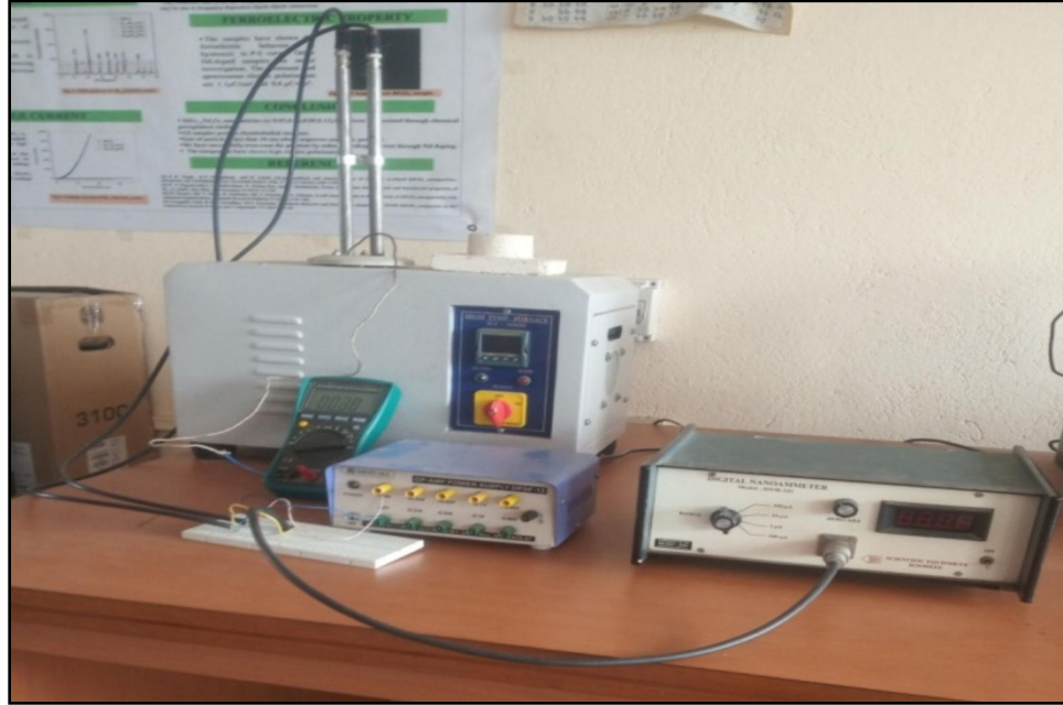
Fig 2.13 Experimental set-up for temperature dependent DC conductivity measurement.
