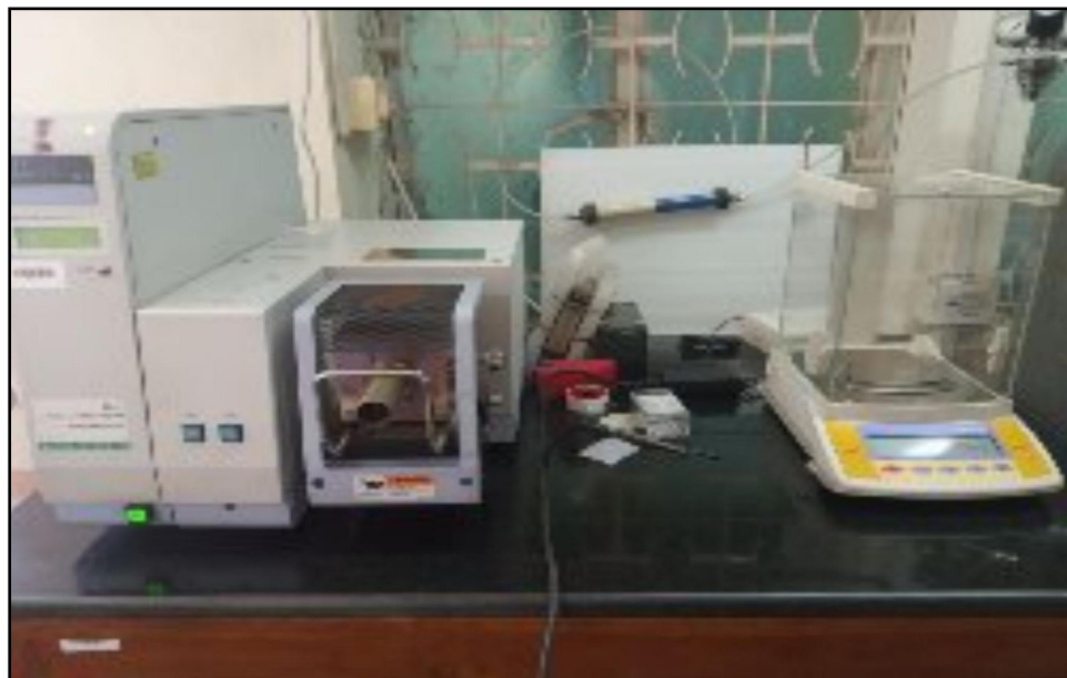
Fig 2.7 Experimental set-up of DTA/TGA.
