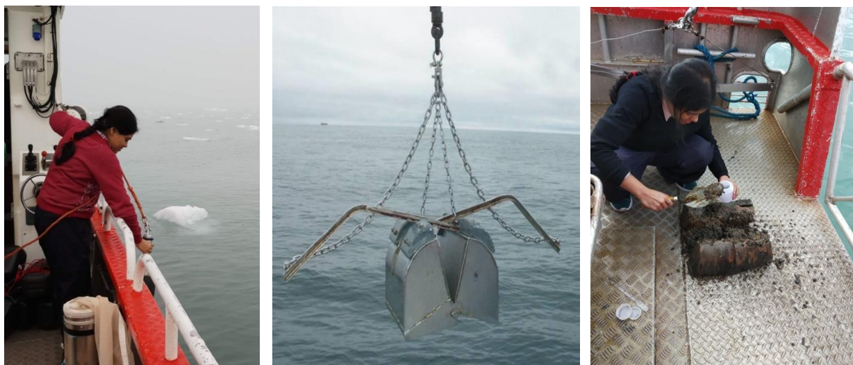
Figure 2.5: Collection of Recent Sediments : [a] CTD measurements, [b] Van Veen grab used for sampling, and [c] Collection of modern samples from Kongsfjorden fjord.
