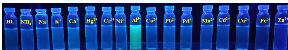
Fig.II.12. In acetonitrile-water (2:1, v/v) of pH, 7.2 (HEPES buffer) UV chamber HL persists color in presence of Al^{3+} but disappears in presence of all other metals.
