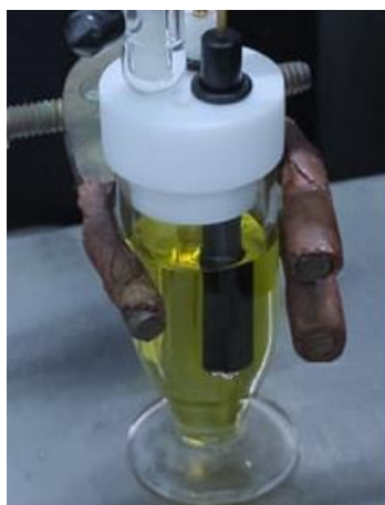
Figure 5.31: Photograph of the customized, one-compartment, three-neck cell with a glassy carbon working electrode. \text{H}_2 gas bubbles are appeared on the surface of the working electrode.
