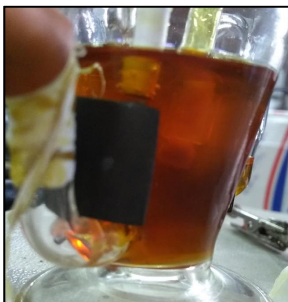
Figure 6.17: Photograph of the customized, one-compartment, three-neck cell with a graphite working electrode containing 0.5 mM of complex 6.1 in air free DMF, 35 mM acetic acid and 0.1 M TBAB as supporting electrolyte. H_2 gas bubbles are appeared on the surface of the working electrode.
