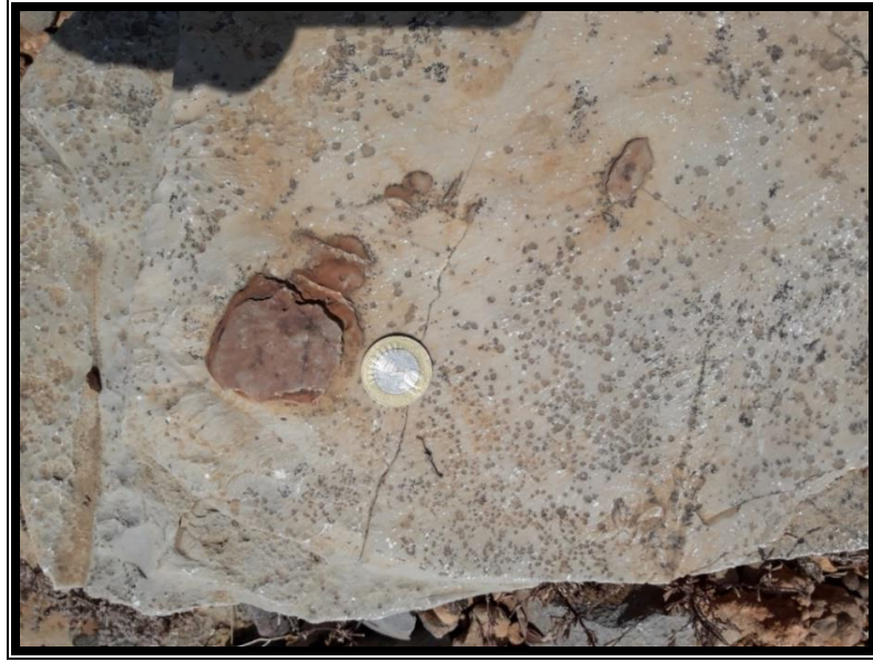
Fig 17. Iron concretion within limestone facies, recorded from Betamcherla area which are mainly formed from oxidation of pyrite. Dimension of the coin - 2.70 cm
