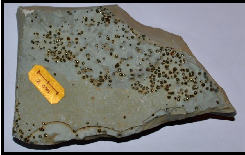
Fig 7. Occurrence of the iron nodules with comparatively larger in size within the Narji limestone, recorded from the Patapadu Yantipalli section.
