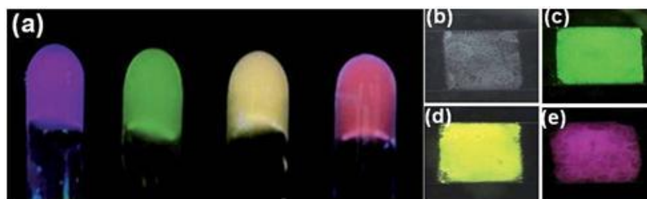
Figure 1.30 (a) Photographs of Lanthanide (III) cholate gels under UV irradiation of 365 nm (from left to right): Eu(III) cholate (5/15 mM) doped with 6mM pyrene, Tb(III) cholate (5/15 mM), Tb(III)–Eu(III) cholate (4.9/0.1/15 mM) and Tb(III)–Eu(III) cholate (4/1/15 mM).
