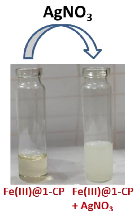
Figure 3.22. AgNO 3 test for presence of Cl - as counter ion in Fe(III)@1-CP .
