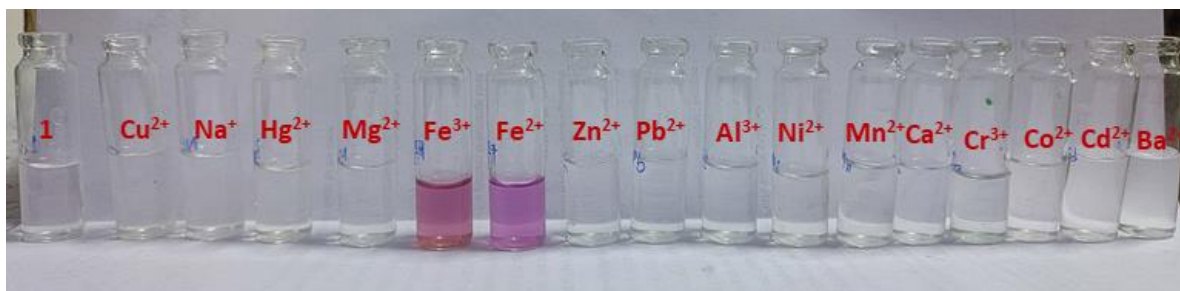
Figure 3.21. Visualization test of Coordination polymer, 1 with different metal ions.
