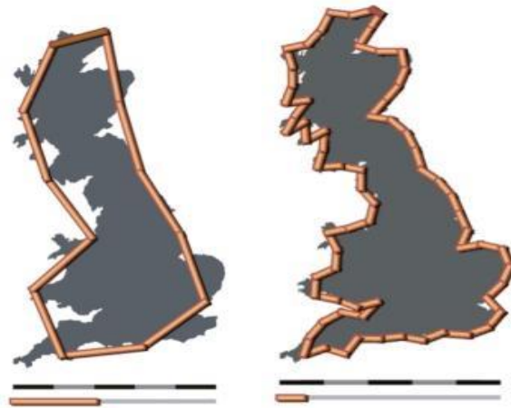
Fig. 1.9.2. The coastline of Britain in different scales: larger (left) and smaller (right)
