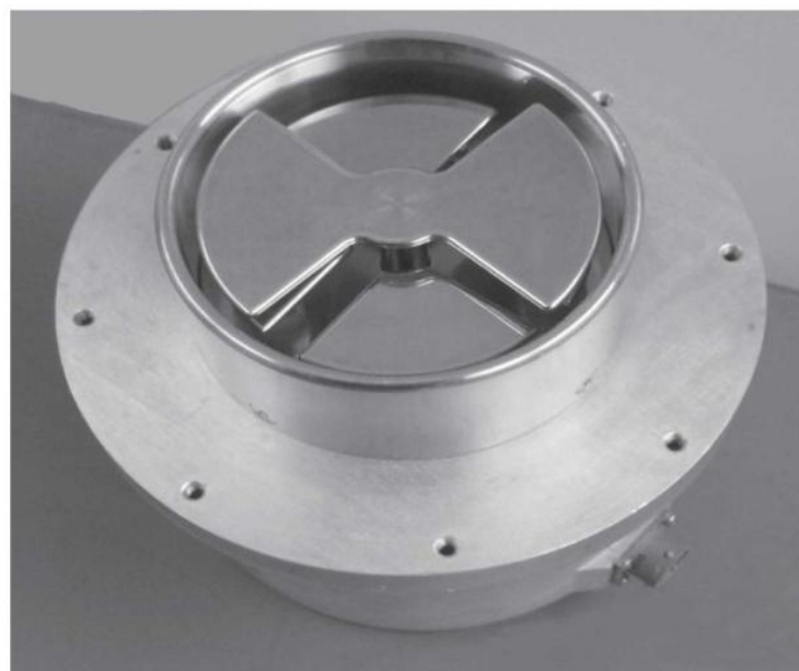
Fig. 2.2: A standard Field mill apparatus that shows the modulator, pressure cover, and electric connector.
