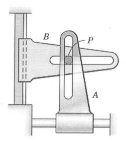
Q1(b) The sphere P travels in a straight line with speed v = 10 m/s. For the instant depicted, determine the corresponding values of  $\dot{r}$  and  $\dot{\theta}$  as measured relative to the fixed Oxy coordinate system. Refer to the following figure.
