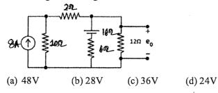
2. In the circuit the power supplied by the voltage source is
